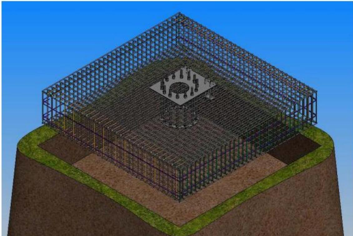
Pad base wired to rebar cage in correct position, and lowered into 4250 x 4250 x 1000 hole. Assembly to be levelled prior to the concrete pour.
